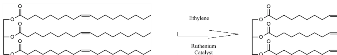
Scheme 3. Cross-metathesis of vegetable oil triglycerides
